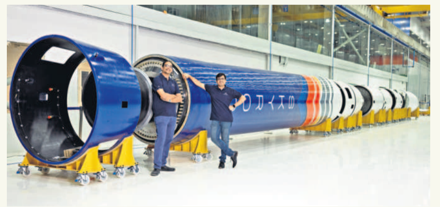
Distinguished by its all-carbon-fibre construction, this rocket can transport multiple satellites into orbit, making it India's first in the space sector and first few globally
